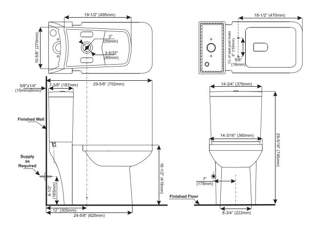
Nominal Dimensions; 29" (737mm) long 14-3/4" (376mm) wide 29-5/16" (745mm) High Water Surface; 8" (203mm) long 6-1/2" (165mm) wide **Trap Passageway;** 2″ (51mm) diameter Fully Glazed
